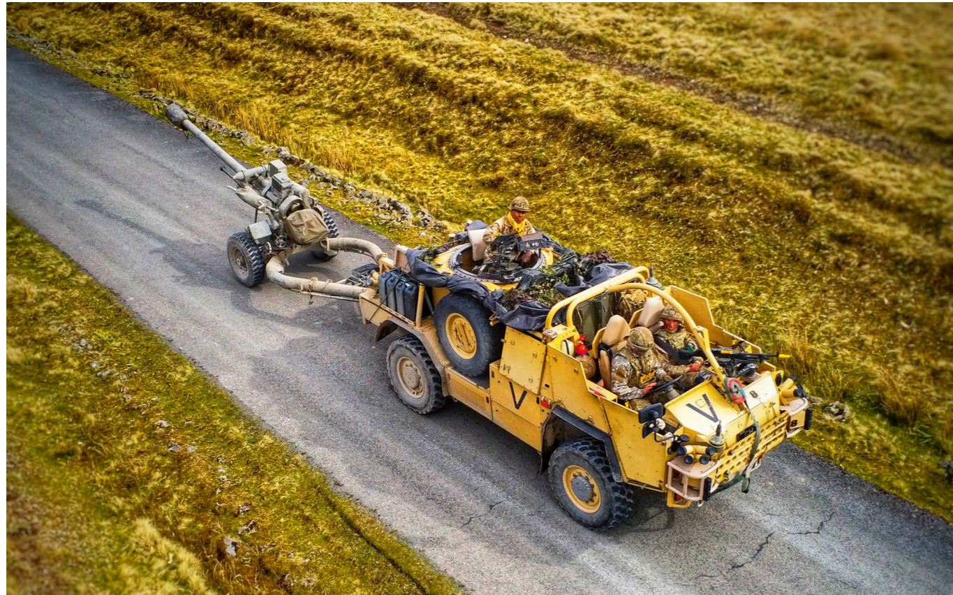
8 (Alma) Cdo Bty using the Jackal as a Gun Towing Vehicle (GTV) on Ex ALMA CANNON.
